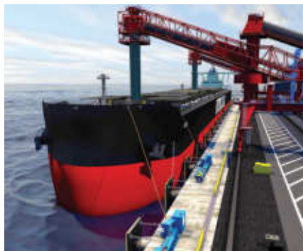
DynaMoor actively maintains tension in mooring lines to dampen vessel movements.
