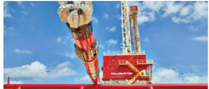
The iCruise X is equipped with an advanced steering head fit for greater durability in operations.
