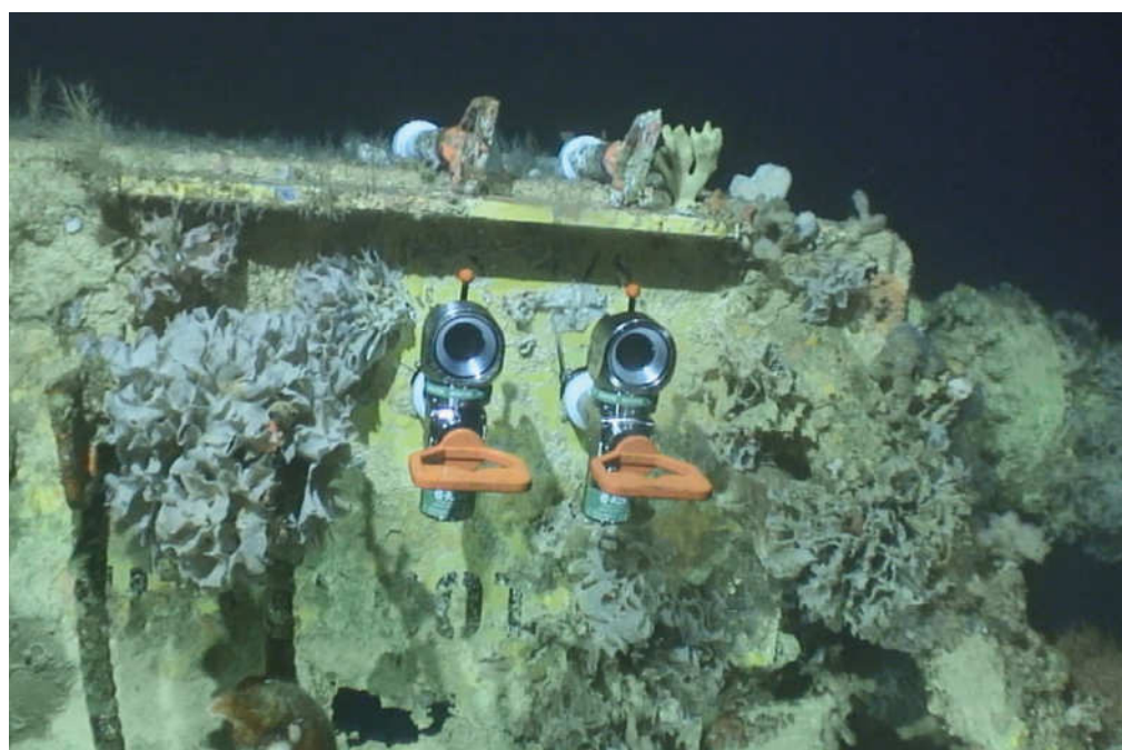
C-Kore units installed subsea.
