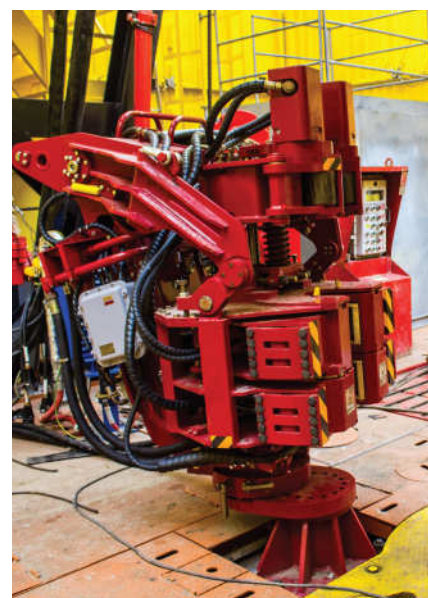
A robot for screwing pipes on the drilling rig.
