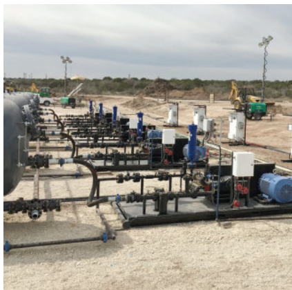
Wanner International Ltd's hydra-cell jet pump hydraulic artificial lift solution.
