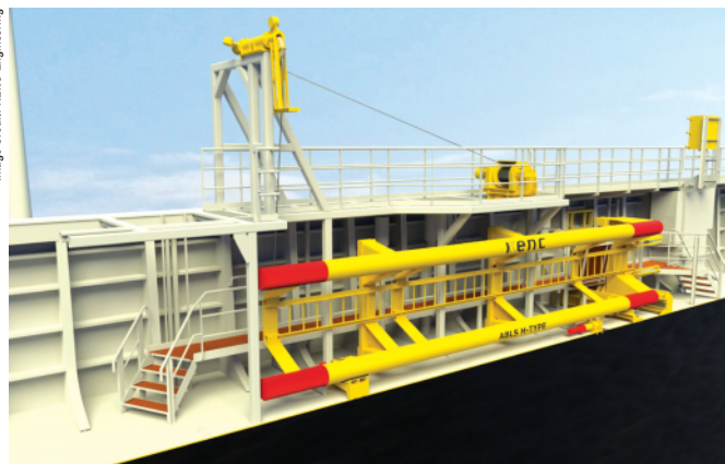
ABLS comes fully equipped with an automated control system and hydraulic drives.
