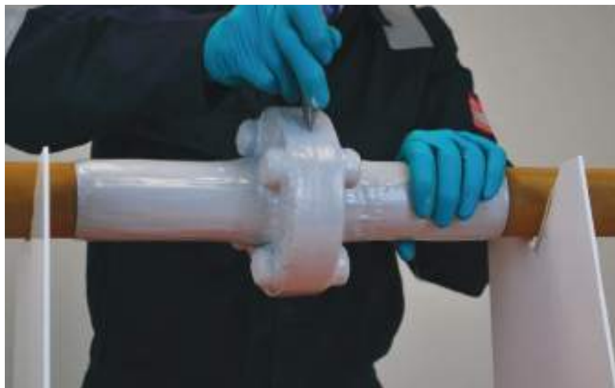
Encapsulating system being cut for inspection.
