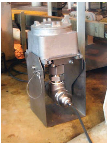
A portable DepCon device, which uses quartz crystal microbalance (QCM) technology to provide real-time optimisation of scale monitoring programmes.
