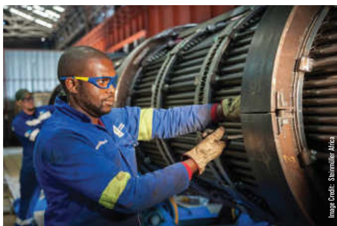
HP Heater Tube bundle final fitments before the shell goes over.
