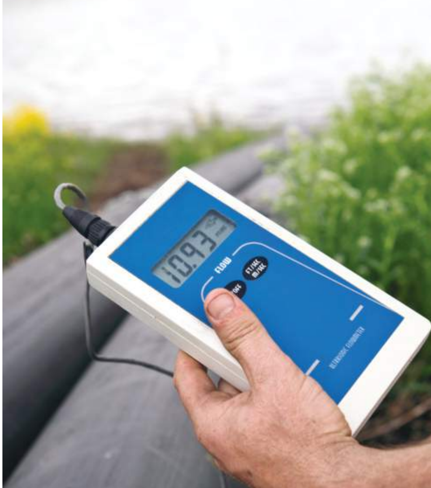
An ultrasonic meter operates on the principle of transit-time.
