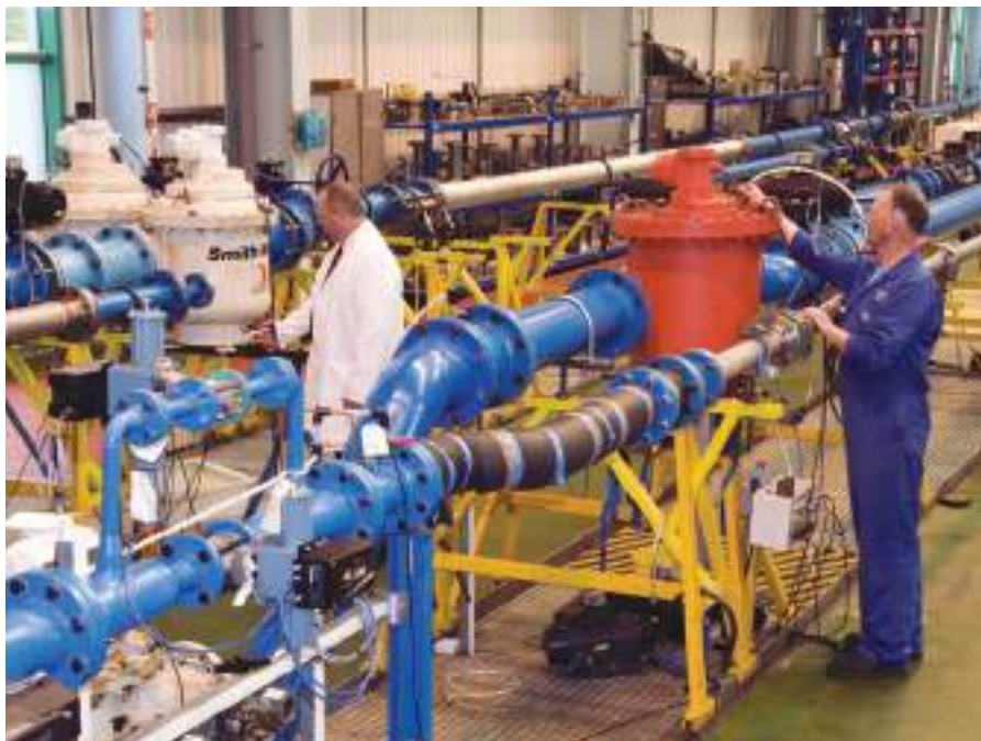
Flow meters being calibrated under laboratory conditions.
