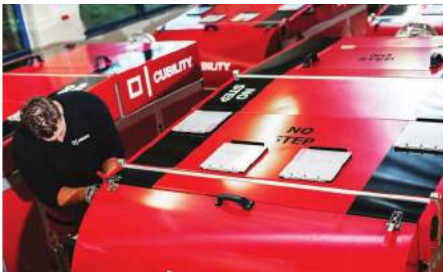
The solids removal efficiency of the MudCube system is said to be as high as 90 per cent.
