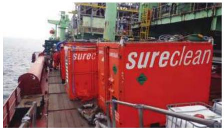
Sureclean's Vacuum Systems were engineered to safely remove sludges over 30m vertically and 100m horizontally from crude oil storage tanks.
