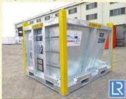
10-TON OMS VACUUM MUD CUTTING SKIP Mfd. to DW 27-1/EN and 8S 12079:2006. • 2213L x 1852W x 1617H Internal Cubic Casacity: 3.7m\* • Payload: 9300kg
