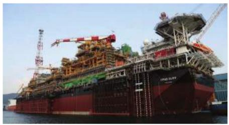
The CLOV FPSO is a giant 119.00-tonne vessel, which can store 1.78mn barrels of oil and is able to process 160,000 bpd.
