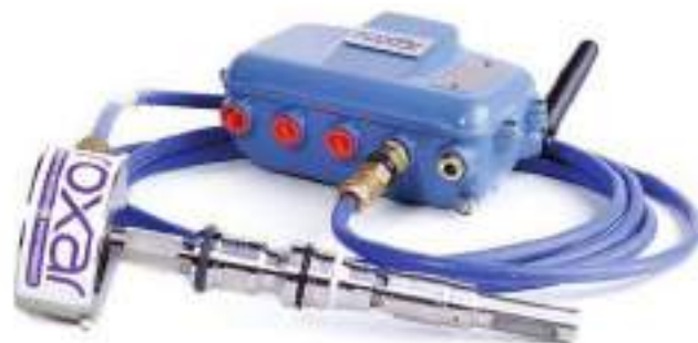
Figure 1 - Emerson's CorrLog wireless corrosion transmitter for ER and LPR probes.
